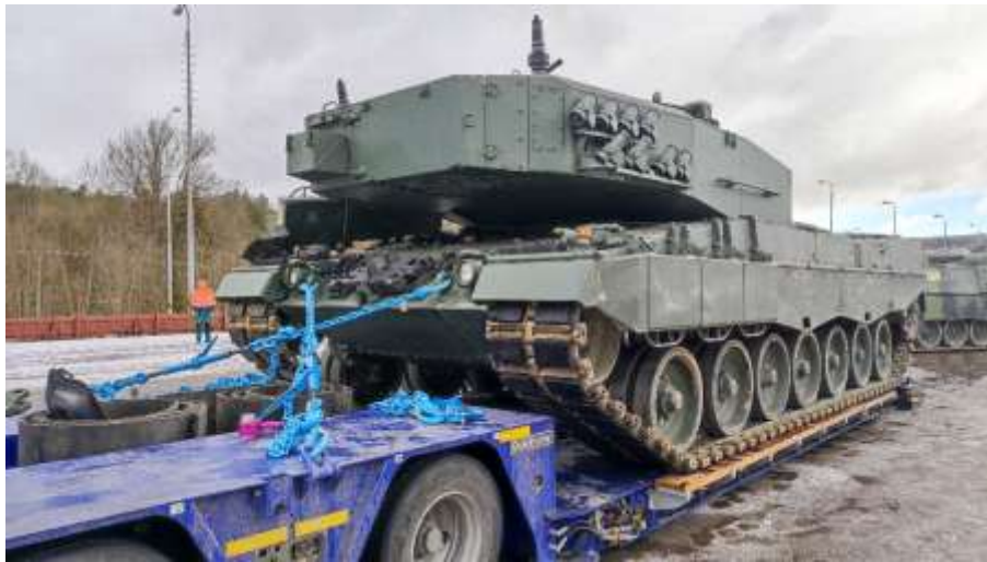
Fig. 1. Rear securing of the Leopard 2A4 tank on a Goldhofer low-bed semi-trailer Photo by the authors
