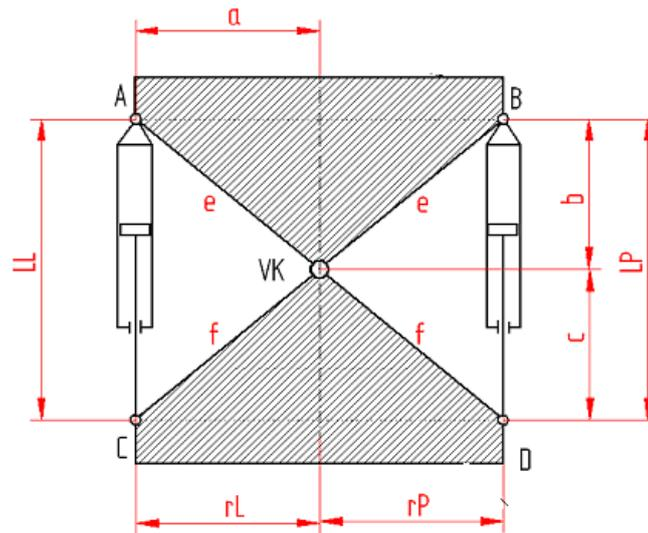
Fig. 2 Scheme of geometric dimensions of a driving mechanism that supports the desired direction of travel
