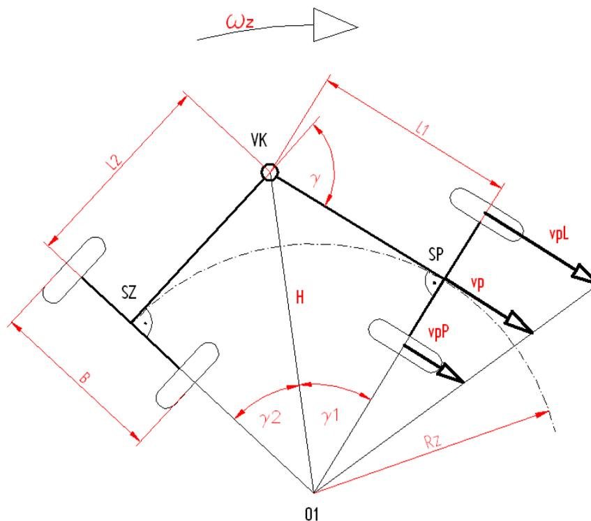
Fig. 3 Curved travel, horizontal projection
