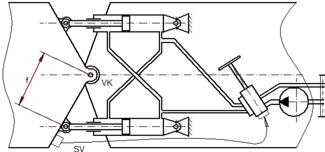
Fig. 1 Scheme of the driving mechanism arrangement
