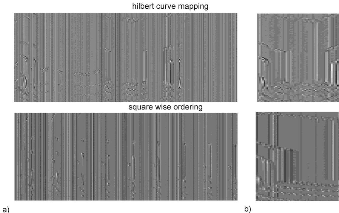
Fig. 4. DWT transforms: a) first 300 coefficients, b) coefficients corresponding to a traffic lane
