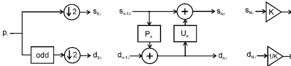
Fig. 1. Lifting scheme steps for computing wavelet coefficients, split, lifting, normalisation
