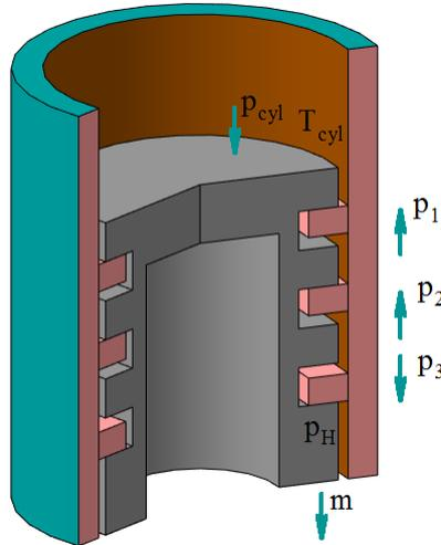
Fig. 5. Case 4 of the positional relationship of the rings in the grooves of the piston, when  $\sum P_1 < 0, \sum P_2 < 0$  and  $\sum P_3 > 0$
