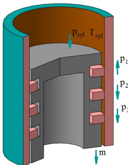
Fig. 2. Case of the positional relationship of the rings in the grooves of the piston, when  $p_{cyl} < p_1 < p_2$  and  $p_2 > p_3$
