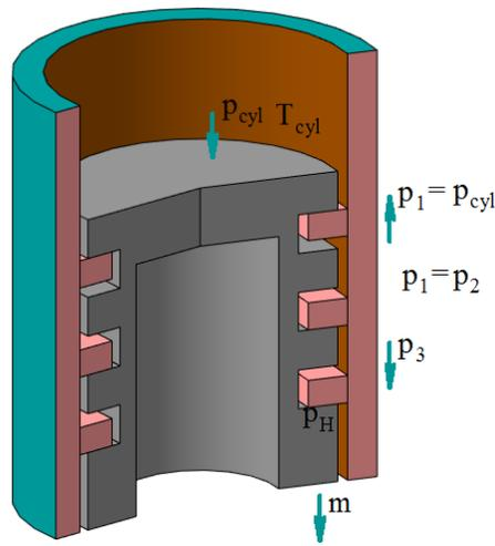
Fig. 7. Case 6 of the positional relationship of the rings in the grooves of the piston, when  $\sum P_1 < 0$ ,  $\sum P_2 < 0$  and  $\sum P_3 > 0$  with  $p_1 < p_2 > p_3$ ,  $p_1 = p_{cyl}$  and  $p_2 = p_1$
