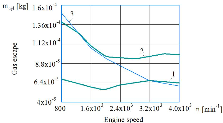
Fig. 9. Changes of the gas escape  $m_{cyl}$  depending on the engine speed: 1 – idling conditions; 2 – load conditions; 3 – the fixed rings
