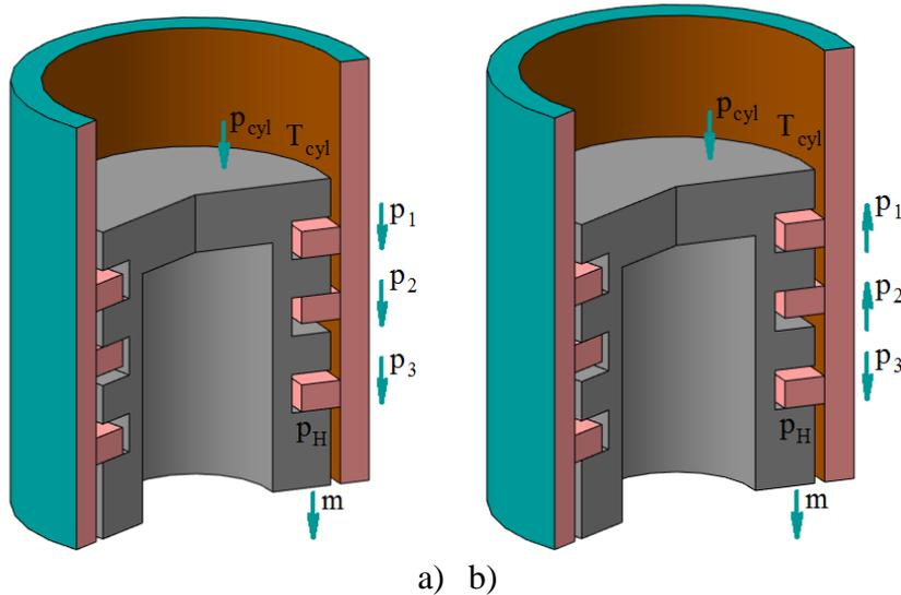
Fig. 4. Case 3 of the positional relationship of the rings in the grooves of the piston, when:
