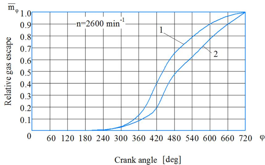
Fig. 8. Changes of the relative gas escape  $\bar{m}(\varphi)$  depending on the crank angle ( $n = 2600 \text{ min}^{-1}$ ) subject to: 1 – the movement of the rings in the grooves; 2 – the fixed rings
