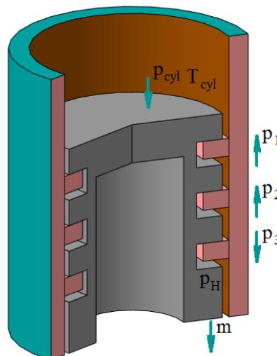
Fig. 6. Case 5 of the positional relationship of the rings in the grooves of the piston, when  $\sum P_1 < 0, \sum P_2 < 0$  and  $\sum P_3 > 0$  with  $p_1 < p_2 > p_3$  and  $p_1 = p_{cyl}$
